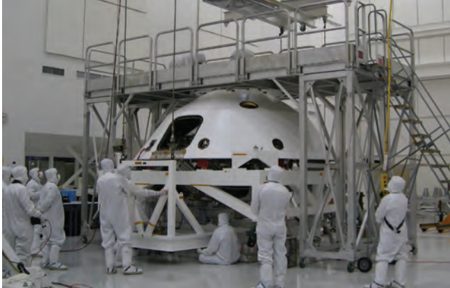
Figure 1. The Entry Vehicle Workstand supports technicians working on the MSL Cruise Stage.
